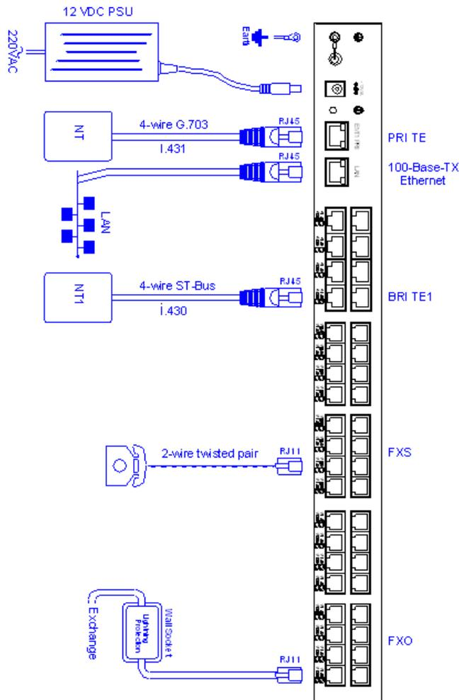
Figure-1: Comma iTA interconnection mechanism
