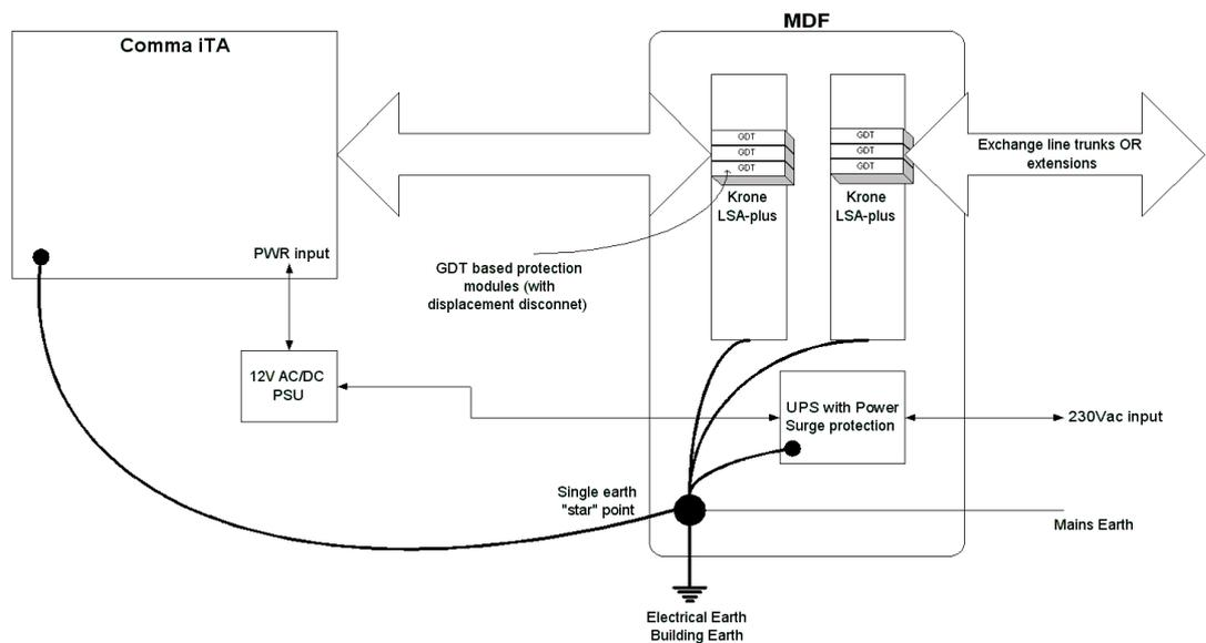
Figure-4: MDF backframe & Comma iTA earth connectivity
